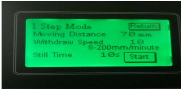
Press on the numbers to select or adjust the Moving Distance, Withdraw Speed and Still Time (The time substrate stays in coating solution).
