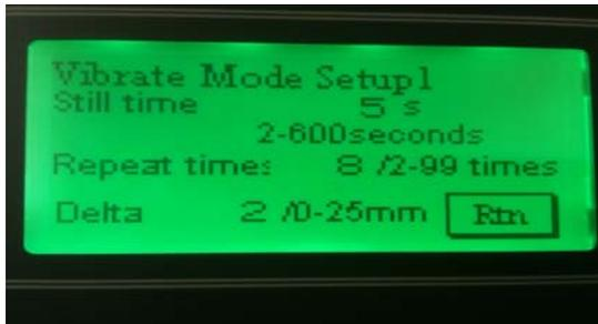
Press "Setup1" to enter the still time or residence time, repeat times or cycles and Delta or the depth difference between each cycle, then press "Rtn" to continue the setup. Press "Setup2" on the Vibrate Mode screen, the following screen will show:
