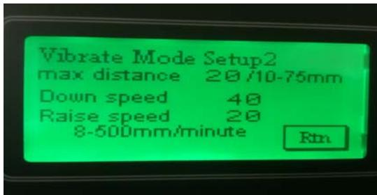
Enter the desired maximum distance or depth, down speed, and raise speed. With the example setup, the very bottom of a substrate will stay in solution for a total of  $5 \text{ sec} \times 8 = 40$  seconds, and the section 18 mm from the bottom will have a residence time of 5 seconds, and so on.
